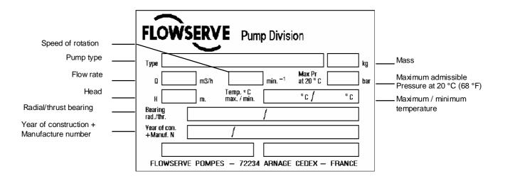
Each pump unit is supplied with the following nameplate:
